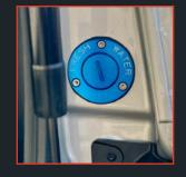
**30L ONBOARD FRESHWATER TANK**- with easy refill point in tailgate
